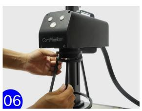
8. Fasten the small ring to fix the auxiliary holder with the right focus
