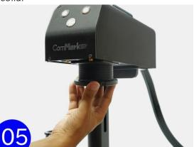
7. Adjust the height of the auxiliary holder according to the focus length
