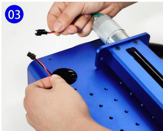
4. Put the motor into the main case
